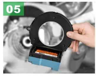
Move steering angle sensor (if any) to NEW clock spring.
