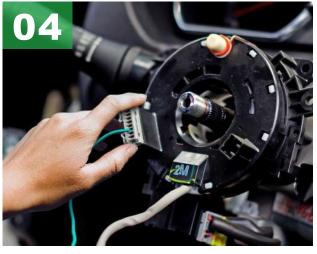
Disconnect cables and remove worn clock spring.
