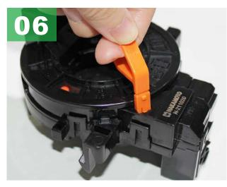
Remove lock pin before installation.
