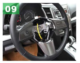
Reconnect airbag module and battery.
