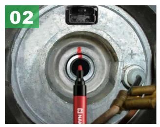
Mark alignment on steering wheel and shaft.
